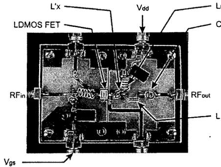
Fig. 5. 200 MHz Class E Power Amplifier Prototype
